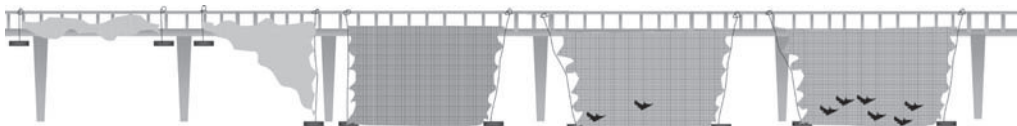
Figure 3. A step by step instruction how to lower a mistnet, using lines and weights. The first step is to attach the lines to the weights and hang them to the bridge. The mistnet is attached to the two lines, opened and the weights are lowered onto the water surface.
